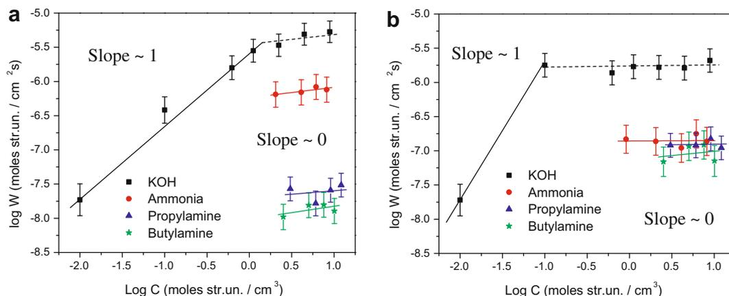
Fig. 1. Log–log plot of reaction rate ( $W$ ) vs. concentration ( $C$ ) for determination of reaction order, for (a)  $Ge_{23}Sb_7S_{70}$  and (b)  $As_2S_3$ .
