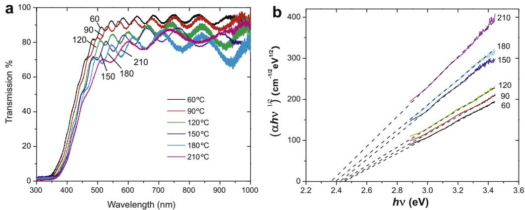
**Fig. 5.** (a) UV-Vis transmission spectra of spin-coated  $\text{Ge}_{23}\text{Sb}_7\text{S}_{70}$  films from propylamine solution with different heat treatment prepared in air. (b) The dependence of  $(\alpha h\nu)^{1/2}$  on photon energy ( $h\nu$ ) in the films from which the effective optical band gap  $E_g^{\text{opt}}$  is estimated (Tauc's extrapolation).
