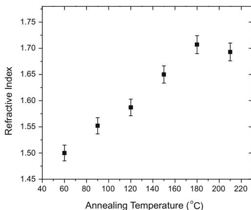
**Fig. 6.** Effect of post-soft bake annealing temperature on refractive index at 680 nm.
