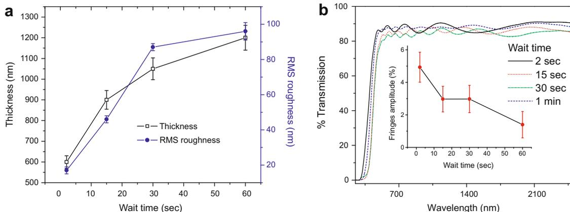
**Fig. 2.** Thickness and roughness measured by Zygo (a) and transmission spectra (b) of films prepared with different wait times prior to spinning; inset: average fringe amplitude.  $Ge_{23}Sb_7S_{70}$  to propylamine ratio 0.5 g/10 mL, stirred for 48 h.
