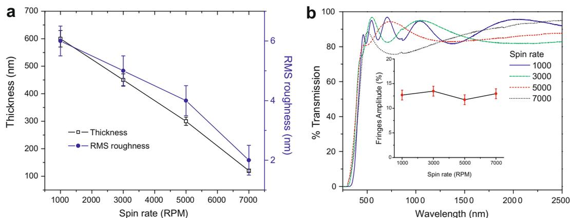
**Fig. 3.** Thickness and roughness measured by Zygo (a) and transmission spectra (b) of films prepared with different spin rates; inset: average fringes amplitude.  $\text{Ge}_{23}\text{Sb}_7\text{S}_{70}$  to propylamine ratio 0.5 g/10 mL, stirred for 48 h.
